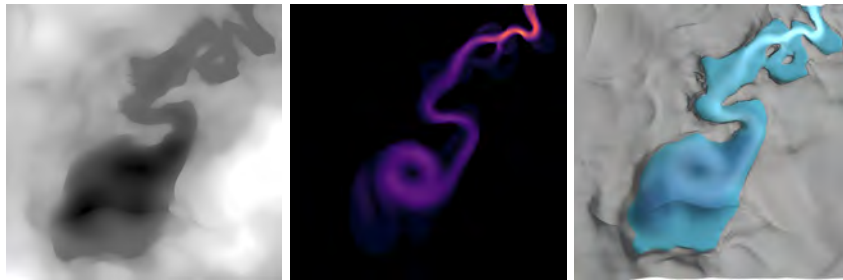
Figure 21.4. Left: terrain height map. The whiter areas indicate higher elevations. Middle: flowmap. The dark purple shades represent lower velocity magnitudes, while the bright yellow shades represent higher velocity magnitudes. Right: top view of the rendered scene.
