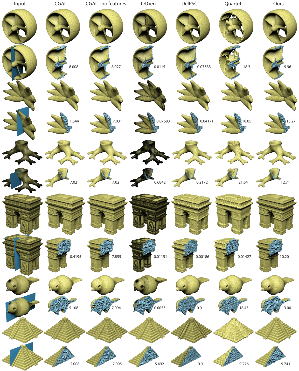
Fig. 15. Comparison with state-of-art tetrahedralization algorithms. The number close to each model is the minimal dihedral angle.
